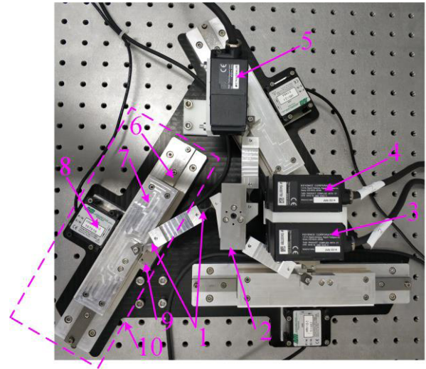
FIGURE 7. The experiment setup of the 3-PRR CPM (1. VTFP; 2. Moving target; 3. Laser displacement sensor-1; 4. Laser displacement sensor-2; 5. Laser displacement sensor-3; 6. Linear guide; 7. Slider; 8. LUSM; 9. Linear encoder; 10 LUSM based linear stage).
